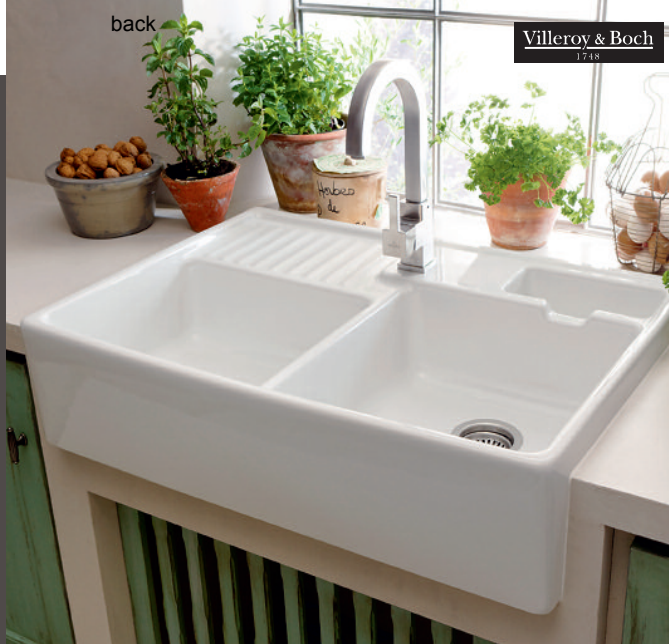
Butler 90 1.75 bowl Ref. 6323 691 R1 AlpineWhite £655 Installation: Bespoke Overall size: 895/630/220 mm Bowl size: 425/420/180 mm Second bowl size: 425/355/180 mm Minimum cabinet size: 900 mm Wastes: 90mm BSW included Tap-Hole: Yes Overflow: Yes
